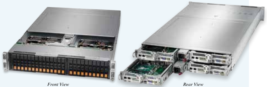
Front View Rear View SYS-2028BT-HTR+ / SYS-2028BT-HNR+ 4 DP Nodes in 2U, 24x 2.5" NVMe/SAS3/SATA3 drives
