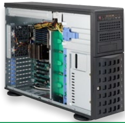
DP Tower/4U Server
