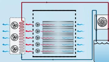
**Rear Door Heat Exchanger** – The rear door of a rack contains several fans that draw hot air away from the servers and cool the air before the air is returned to the datacenter. The cooling liquid is then chilled externally to the door.
