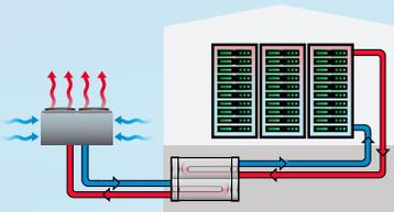
**Direct To Chip** – Liquid passes directly on the surface of a chip and draws heat away. The liquid is then cooled through a liquid to liquid heat exchanger, either contained within the rack or externally.
