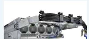
The Cable Management Arm is integrated into the rack mounting rails, included with the top-loading systems, allowing for easy Hot-swap serviceability of the drive bays.
